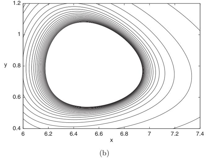
Fig. 3. Simulation results of system (7) for  $d = 0.012$ ,  $a = 0.93$ ,  $c = 40$ ,  $b = p = q = 5.6$ ,  $\eta = 0.01$ , with the initial condition,  $x(0) = 5.0$ ,  $y(0) = 1.0$ ,  $z(0) = 2.0$ ,  $v(0) = 0.5$ ,  $w(0) = 4.0$ : (a) time history showing convergence to a stable periodic solution; (b) phase portrait projected on  $x$ - $y$  plane indicating a stable limit cycle.
