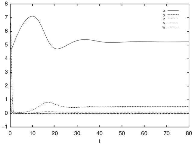
Fig. 2. Simulated time history of system (7) for  $d = 0.04$ ,  $a = 0.93$ ,  $c = 40$ ,  $b = p = q = 5.6$ ,  $\eta = 0.01$ , with the initial condition:  $x(0) = 5.0$ ,  $y(0) = 1.0$ ,  $z(0) = 2.0$ ,  $v(0) = 0.5$ ,  $w(0) = 4.0$ , converging to the stable equilibrium solution  $E_d^\eta$ .
