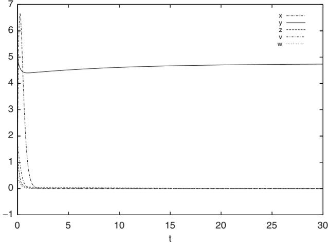
Fig. 1. Simulated time history of system (7) for  $d = 0.21$ ,  $a = 0.93$ ,  $c = 40$ ,  $b = p = q = 5.6$ ,  $\eta = 0.01$ , with the initial condition:  $x(0) = 5.0$ ,  $y(0) = 1.0$ ,  $z(0) = 2.0$ ,  $v(0) = 0.5$ ,  $w(0) = 4.0$ , converging to the stable equilibrium solution  $E_0^\eta$ .
