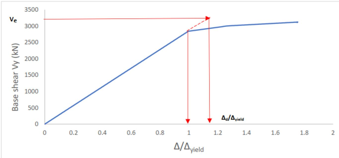
Pushover Load-Displacement Curve for I-Section Shear Wall
