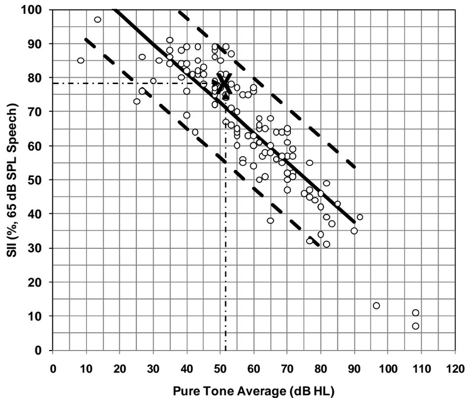
**Figure 5:** Aided SII Normative Values graph with the SII value for a moderate level speech input from the fitting in Figure 3 above. The child has a pure tone average (PTA) of 52 dB HL and the SII value for a 65 dB SPL speech input was measured to be 78%. Therefore, the X represents the intersection of PTA and SII for this fitting. Note that the X falls within the dashed lines indicating it is an acceptable fitting for this child’s PTA.
