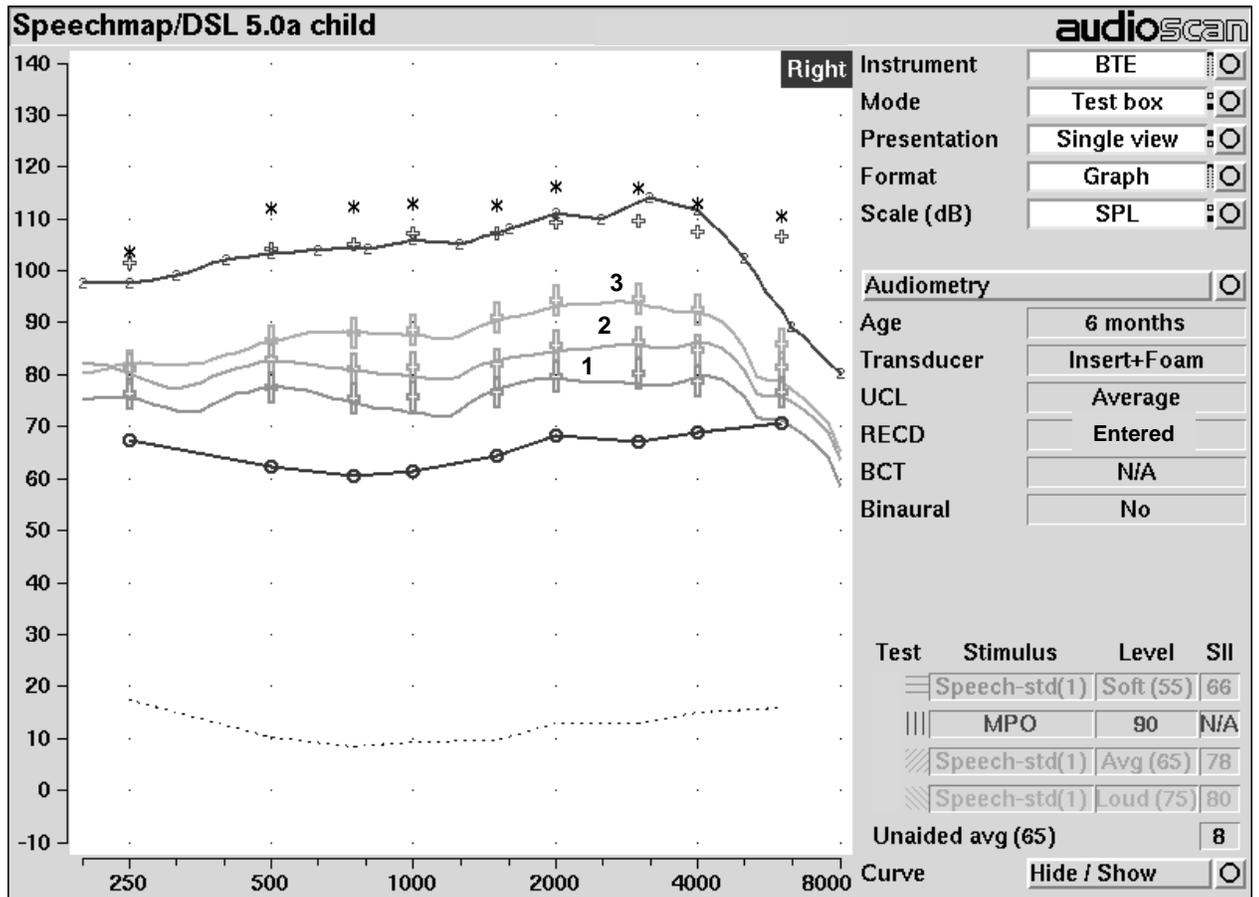
**Figure 3:** SPLogram display of hearing instrument performance in relation to pediatric DSL *m*[i/o] v5.0a targets for a child with a PTA of 52 dB HL. The solid lines represent the output of the hearing instrument for soft (1), average (2), loud (3) speech inputs and MPO (4) in relation to the various speech targets (large +) and MPO targets (small +). Thresholds (o) and upper limits of comfort (\*) are also displayed.
