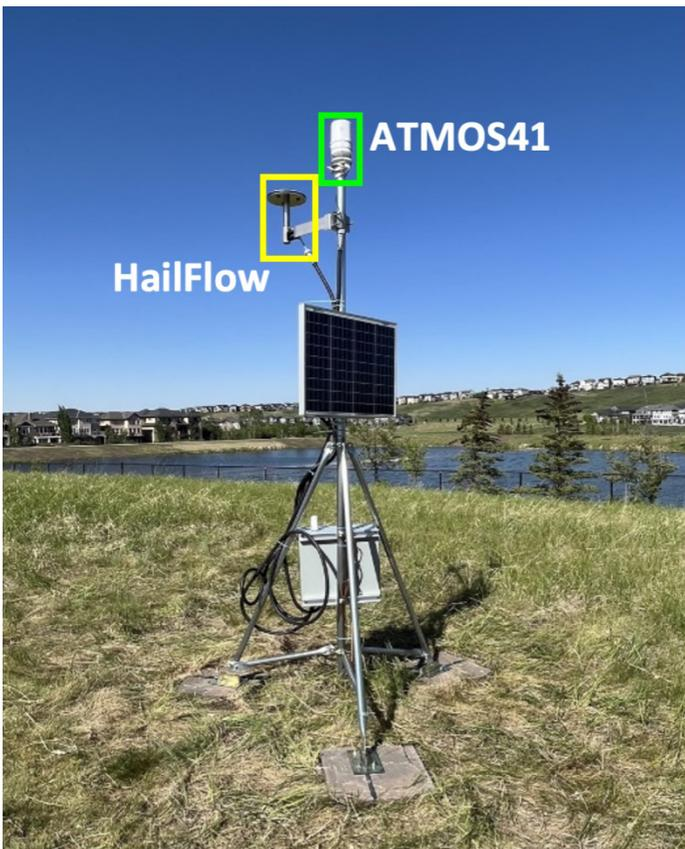
Figure 12: One of the hail-monitoring stations (located at Symons Valley) in the Calgary network. See text for details.
