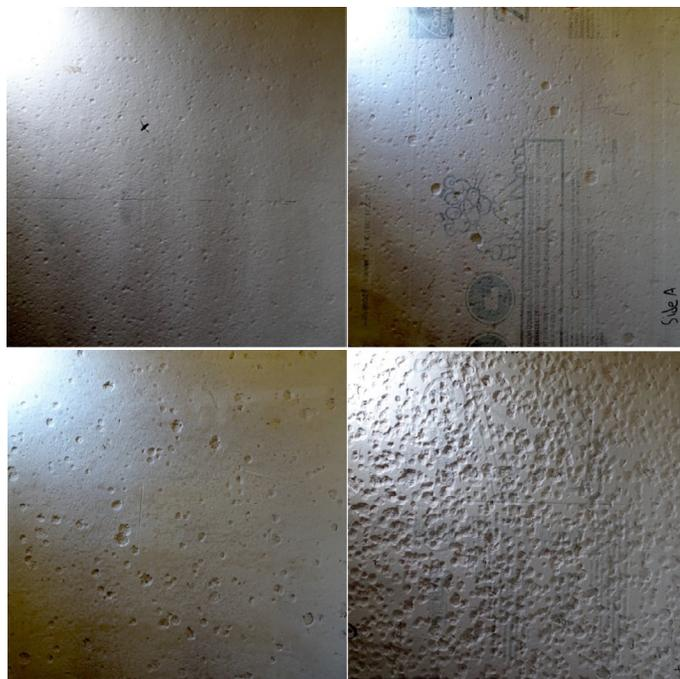
Figure 19: Examples of hailpads hit by hail in 2023. (TL) Large number of small hailstones (~5-7 mm), (TR) Some larger stones (10-15 mm) mixed with many small hailstones, (BL) Random assortment of 10-15 mm hailstones, (BR) A "saturated" hailpad that was hit by many hailstones, some of which were severe.
