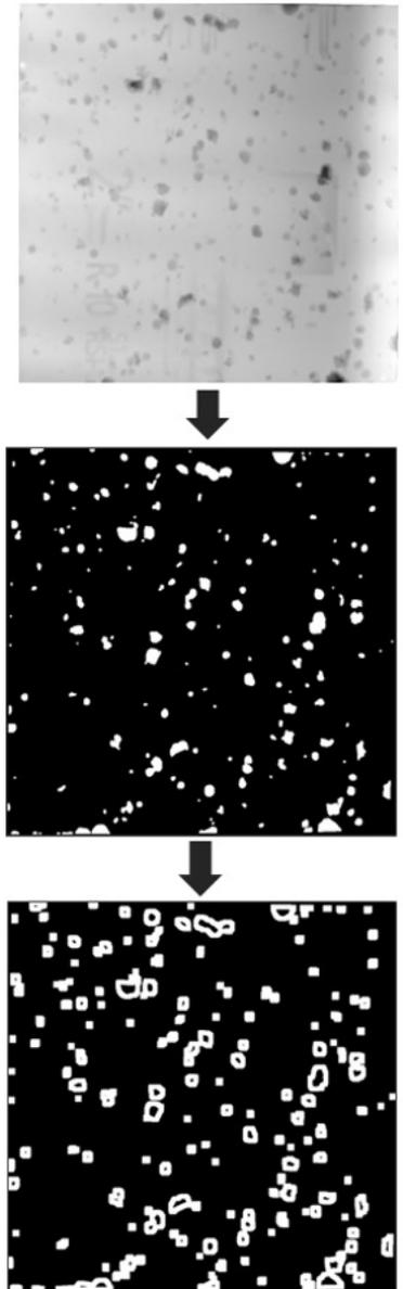
Figure 25a: (top) Preliminary analysis of a test hailpad. The image begins as a rendering from a 3D laser scan. It is processed to identify dents, and refined using a depth threshold to remove noise. Lastly, a watershed algorithm is applied.
