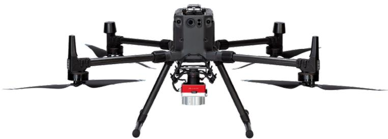
Figure 5: DJI M300 UAV with multi-spectral camera.
