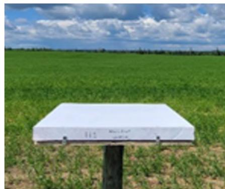
Figure 17: Example of a hailpad deployed in the network.
