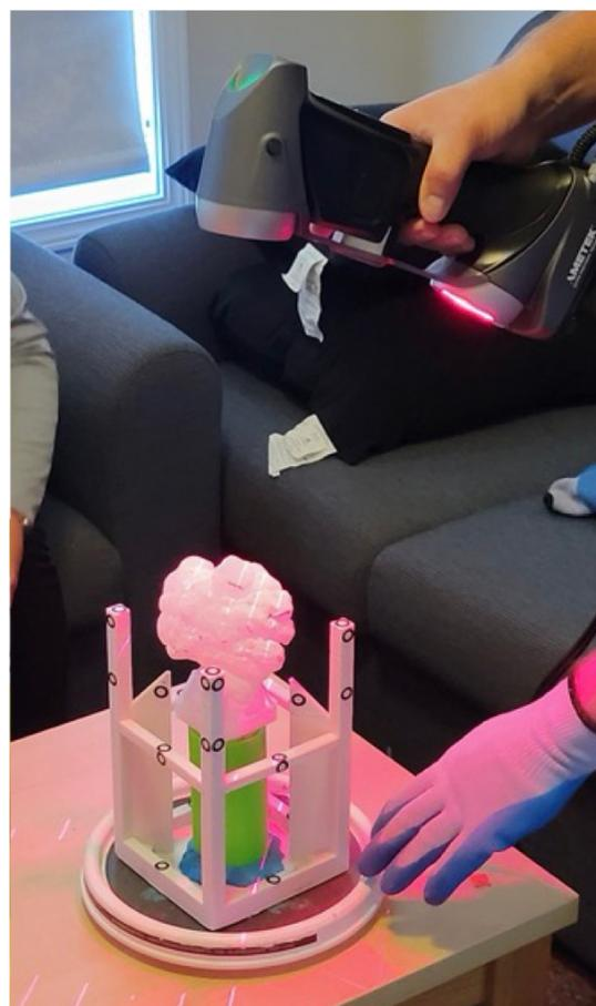
Figure 4: The Markerville, AB hailstone being scanned by the team from IBHS.
